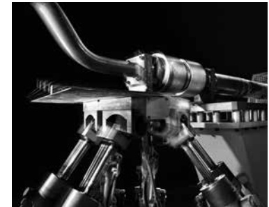
Fig. 2.5 Vibration test bench for simulation of complex application conditions
