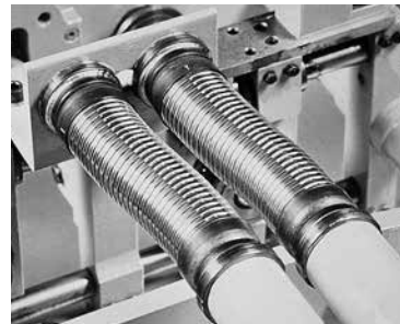
Fig. 2.6 Alternating bending machines for determining the fatigue behaviour of thin strips and sheets
