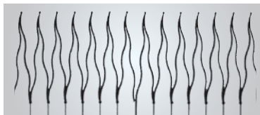
Fig. 3.9 Diaphragms, extremely flexible
