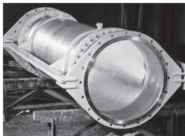
(Fig. 8.25) Lateral expansion joint for paper machines
