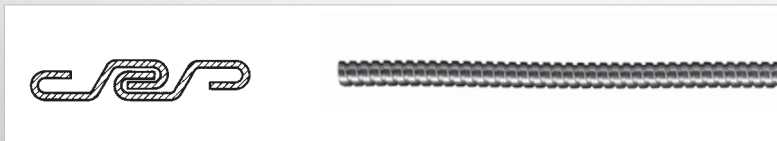
Fig. 2.6.4 stripwound hose with integrated profile
