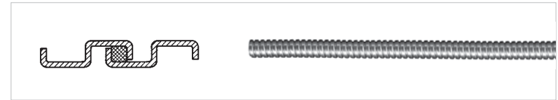
Fig. 2.6.5 stripwound hose with sealing thread
