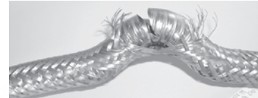
Fig. 4.1.2 Braiding failure and resulting ruptured hose
