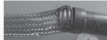
Fig. 4.1.3 Braiding failure at the interface to the end pants
