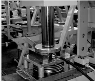
Figure 5.2.1.: Pressure resistance testing on a metal bellows.
