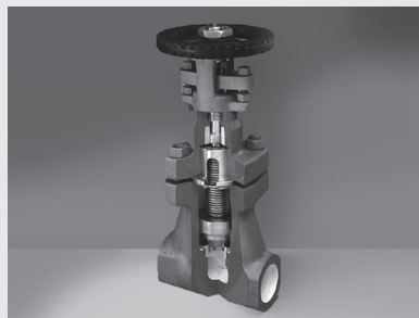
Figure 3.1.1.: Valve with metal bellows as shaft sealing
