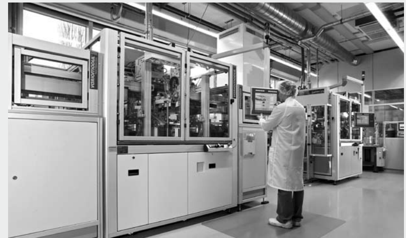
Figure 2.2.2.: HYDRA precision bellows production under clean-room conditions
