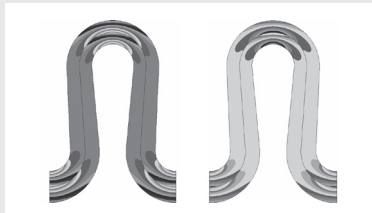
Figure 4.2.1.: Meridional stress on a two-layer metal bellows at axial tension (left) and outside pressure (right)
