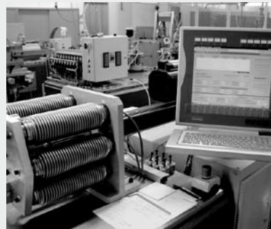
Figure 5.2.2.: Axial load cycle test.
